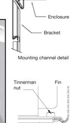
Cutaway view of FF5 enclosure showing  $4 \frac{1}{4}$ " x 4  $\frac{1}{4}$ " fin configuration.
