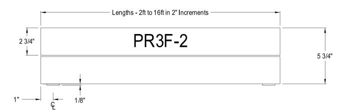
ALL PR3F UNITS PROVIDED WITH SUPPLY CONNECTION ON FRONT HEADER AND RETURN CONNECTION ON REAR HEADER.
