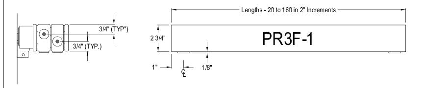
ALL PR3F UNITS PROVIDED WITH SUPPLY CONNECTION ON FRONT HEADER AND RETURN CONNECTION ON REAR HEADER.
