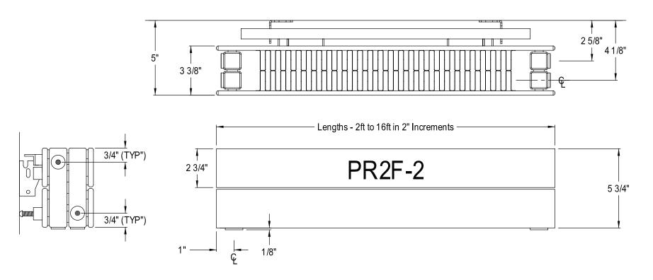
ALL PR2F UNITS PROVIDED WITH SUPPLY CONNECTION ON FRONT HEADER AND RETURN CONNECTION ON REAR HEADER.
