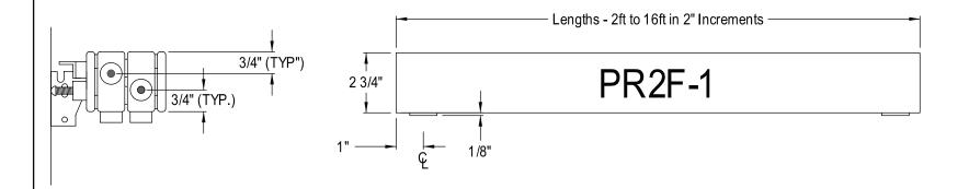
ALL PR2F UNITS PROVIDED WITH SUPPLY CONNECTION ON FRONT HEADER AND RETURN CONNECTION ON REAR HEADER.
