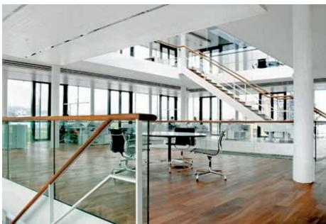
It was mastered through the use of Zehnder radiant ceiling panels: harmoniously integrated on all three floors in the modern geometric architecture, they also ensure that the cold air descending along the glass front panels is considerably reduced.
