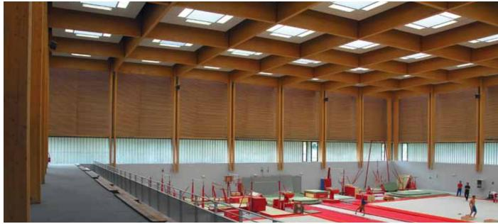
The 12,000 m² of the building have been fitted with Zehnder radiant ceiling panels which build a frame around the lighting. A total of 1,836 m² blends perfectly into the idiosyncratic architecture.
