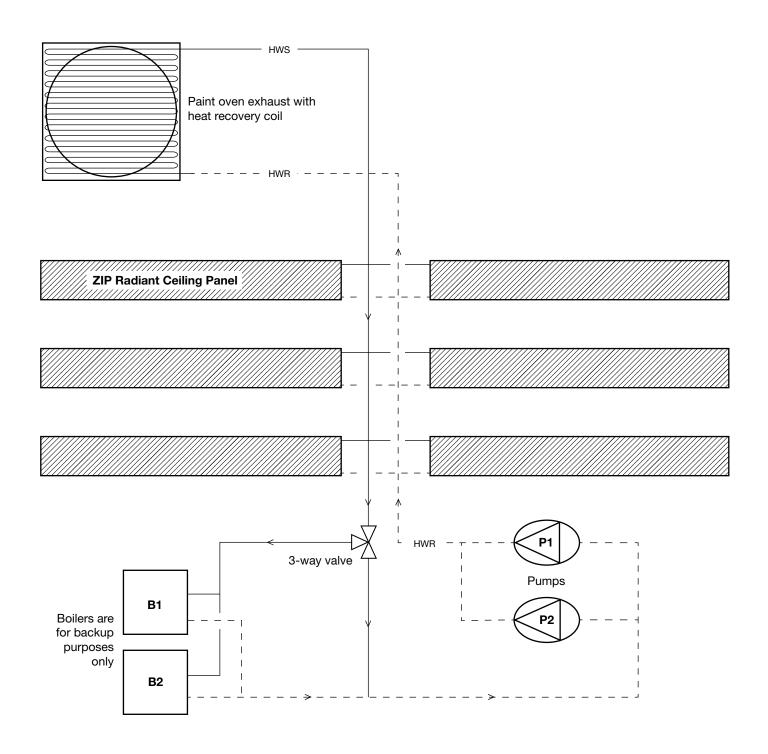
Boilers run 3 hours per day on weekends between November and March, but only when the plant is closed and the waste process heat from the paint line bake oven is not available. The boilers also run about 6 hours per year for routine maintenance.
