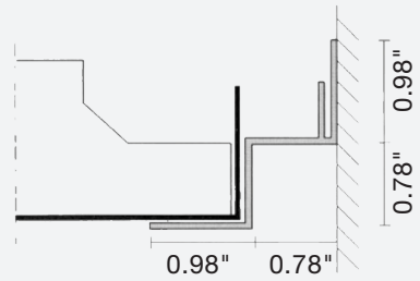
Graded-edge angle for installed inactive panels (Fig. 3)
