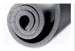
Flexible, elastomeric thermal insulation, black in color. It is furnished with a smooth skin on one side which forms the outer exposed insulation surface. It is manufactured without the use of CFC's, HCFC's, or HFC's. It is also formaldehyde-free, low VOCs, dust free, fiber free and resists mold and mildew.
