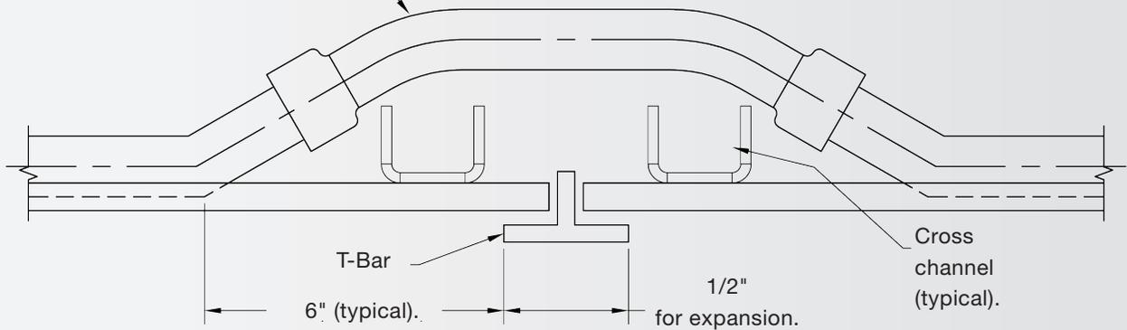
Flexible connections are used between panels when they are installed in series in the same room.
