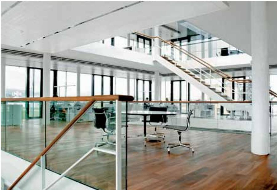
It was mastered through the use of Zehnder radiant ceiling panels: harmoniously integrated on all three floors in the modern geometric architecture, they also ensure that the cold air descending along the glass front panels is considerably reduced.
