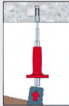
Expand anchor until marking on flared end
