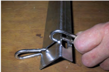
4. Connect snap hook with chain to the multiple suspension bar.
