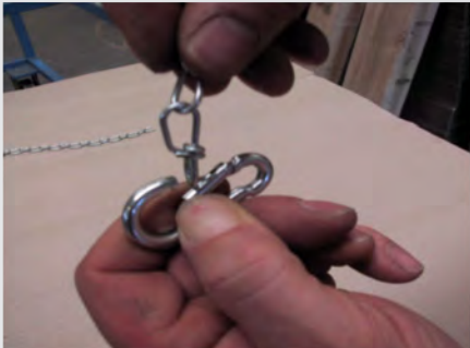
3. Connect snap hook to the chain.
