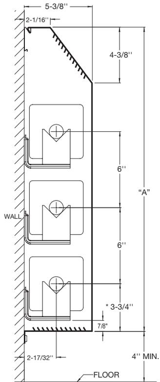
\* CENTERLINES ARE BASED ON 1" COPPER TUBE
