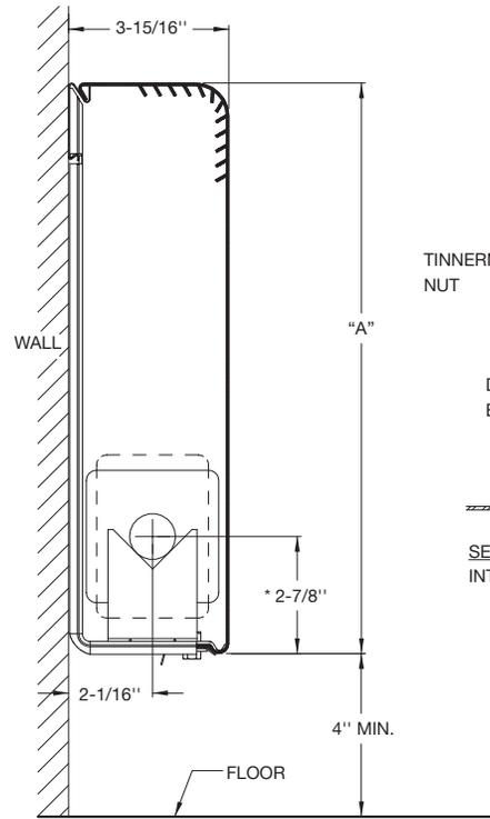
\* CENTERLINES BASED ON 1" COPPER TUBE
