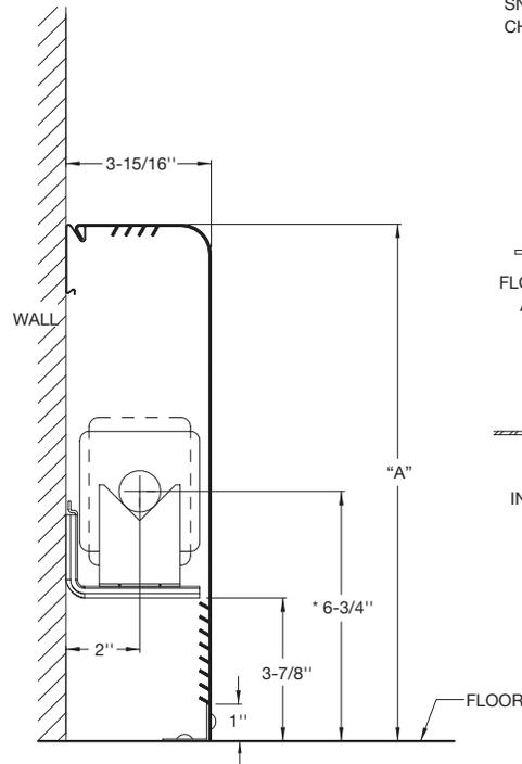
\* CENTERLINES ARE BASED ON 1" COPPER TUBE
