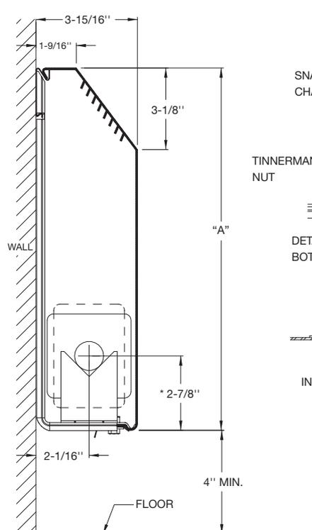
\* CENTERLINES ARE BASED ON 1" COPPER TUBE
