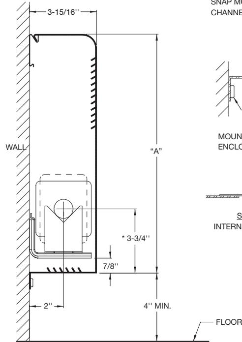
\* CENTERLINES ARE BASED ON 1" COPPER TUBE
