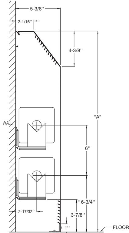
\* CENTERLINES ARE BASED ON 1" COPPER TUBE
