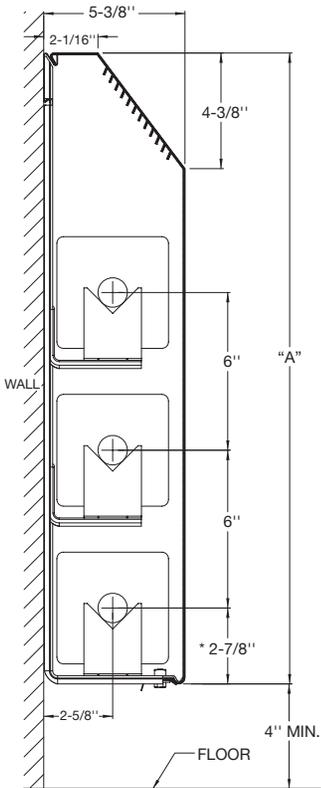
\* CENTERLINES ARE BASED ON 1" COPPER TUBE
