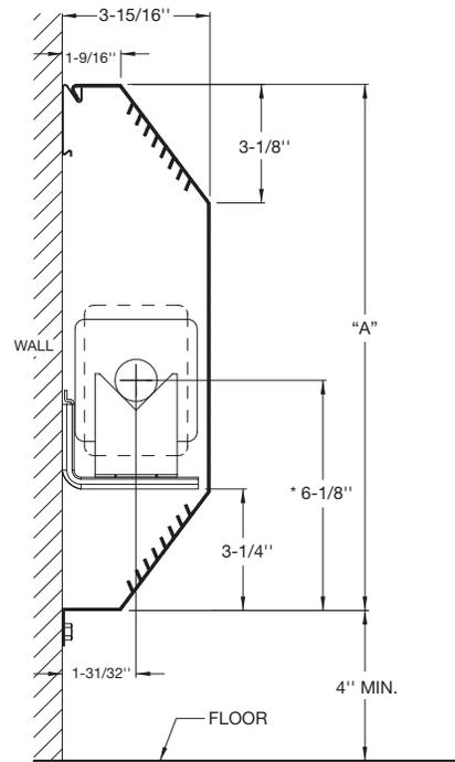
\* CENTERLINES ARE BASED ON 1" COPPER TUBE
