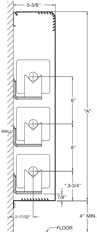
\* CENTERLINES BASED ON 1" COPPER TUBE
