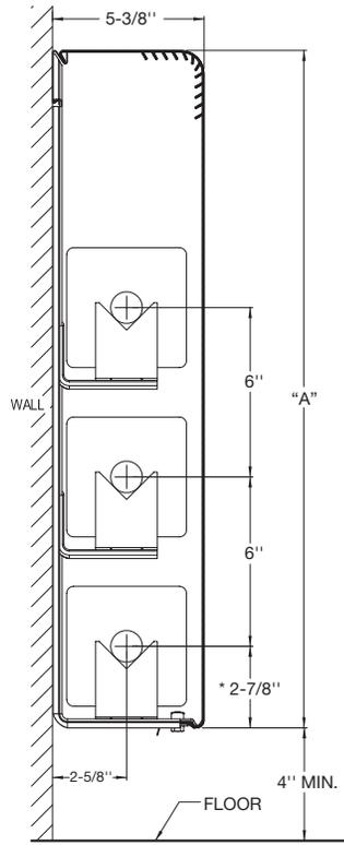
\* CENTERLINES BASED ON 1" COPPER TUBE
