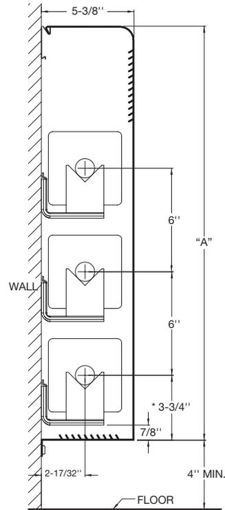
\* CENTERLINES ARE BASED ON 1" COPPER TUBE
