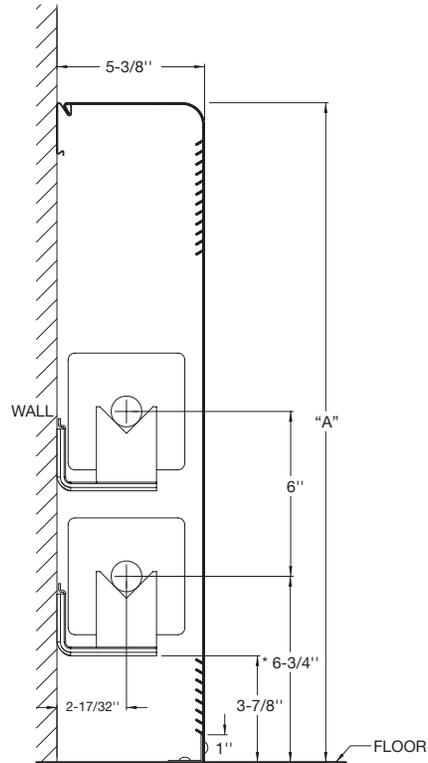
\* CENTERLINES BASED ON 1" COPPER TUBE
