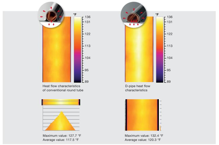
The thermograph shows that the D-pipe produces a more even and more pronounced thermal transfer than a conventional round tube. This is achieved thanks to better encapsulation of the pipe in the aluminium profile and on account of the large contact area of the pipe on the heating and cooling module. With the combination of the D-pipes and the aluminium profiles, a performance increase of 5% is possible depending on heat flow and application.
