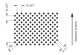
The Zehnder Alumline radiant ceiling panels can be perforated to provide optimized sound absorption. Sound waves pass through the perforations and are absorbed by the specially developed sound insulation. With sails, the sound waves are also absorbed by means of reverberation on the top of the product. This significantly reduces noise and the associated vibrations, especially in openplan offices, call centers, schools, etc.
