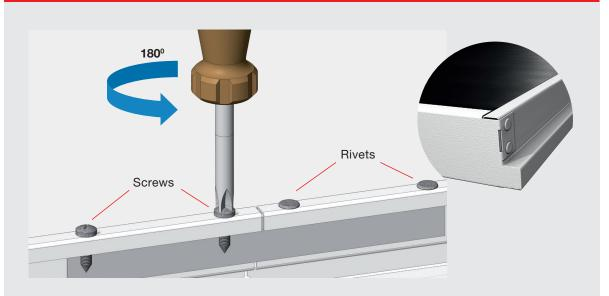
The Zehnder Alumline lay-in modules for grid ceilings are produced from a length of 5' with anti-flec technology. This ensures an even contact surface on the ceiling grid, even when heating at high temperatures. After laying the modules in the grid, the antiflec profiles are loosened in the ceiling grid by opening the screw pairs.
