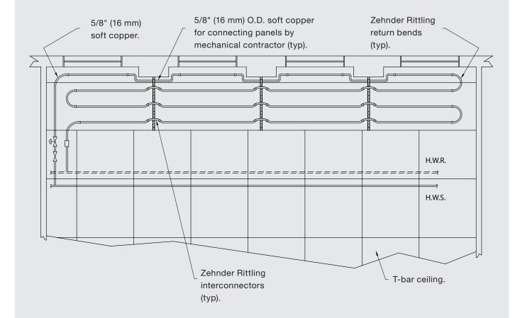
Zehnder Rittling Radiant Panels notched around perimeter columns. Even pass coiling shown.
