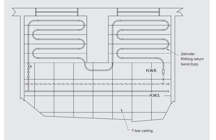
Two odd number pass panels piped, around column.
