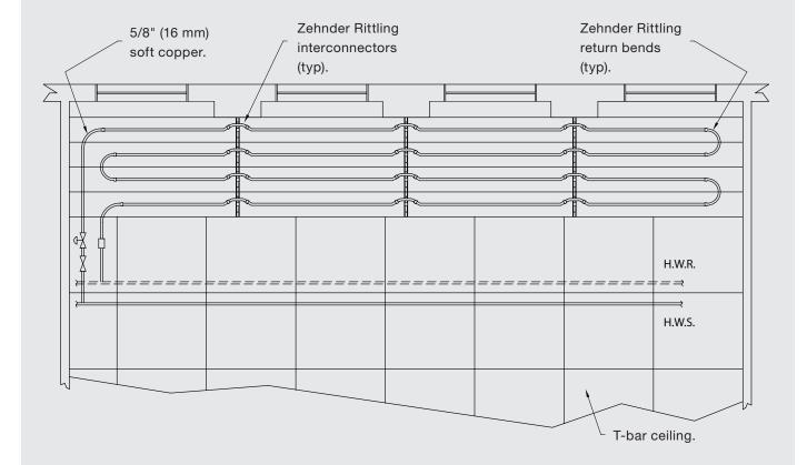
Zehnder Rittling Radiant Panels positioned clear of perimeter columns. Even pass coiling shown.
